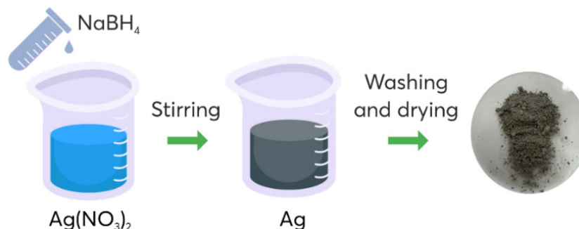
Figure 2. Synthesis of the silver particles. Created with Corel DRAW Graphics Suite 2020.
